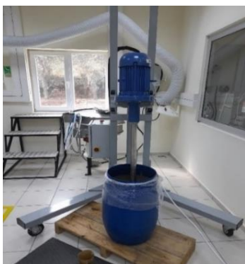
Figure 1. Ultra-Turrax homogenizer (UTC 115kt)
