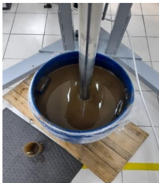
Figure 1. Ultra-Turrax homogenizer (UTC 115kt)
